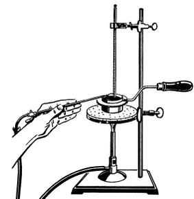
Figure 7. Flash point test
