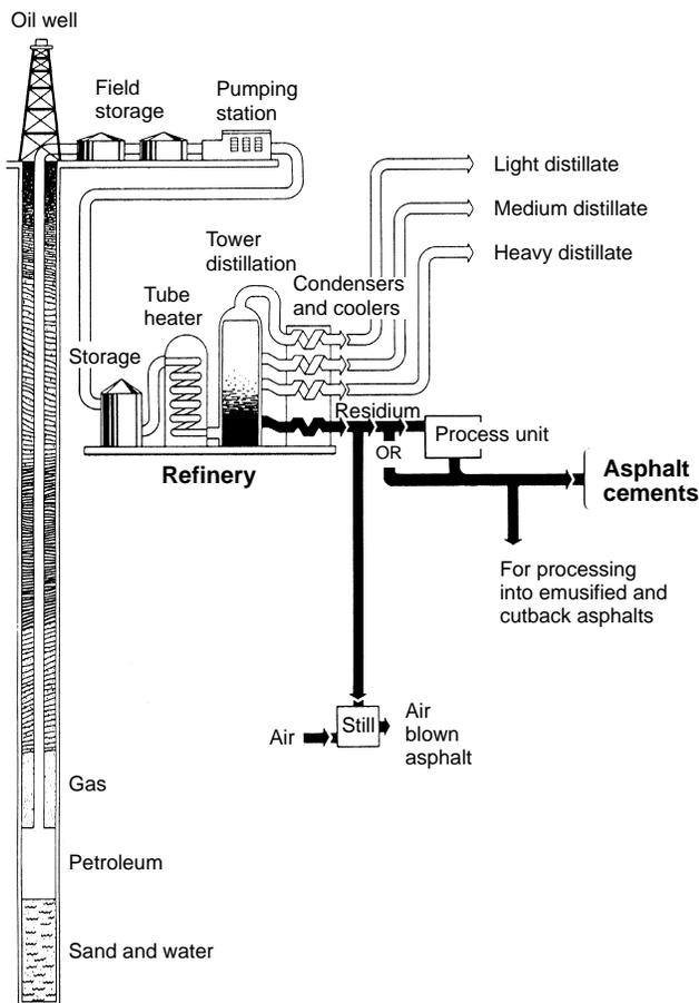
Figure 1. Production of asphalts from refining petroleum crudes
