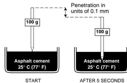
Figure 6. Penetration test
