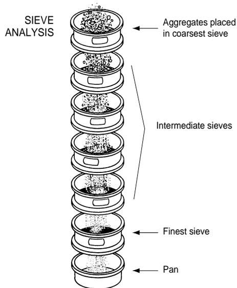
**Figure 4. Determining size and gradation of aggregates**
