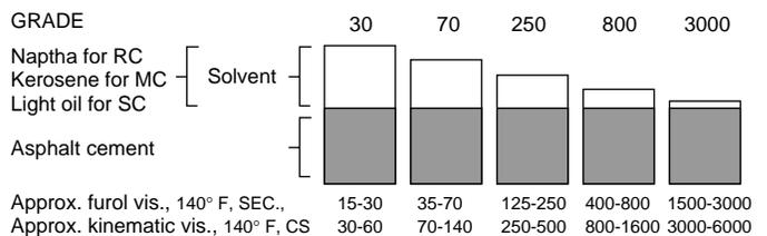
**Figure 3. Composition of cutback asphalts**
