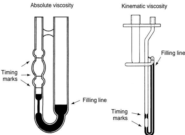
Figure 5. Viscometers for asphalt cement
