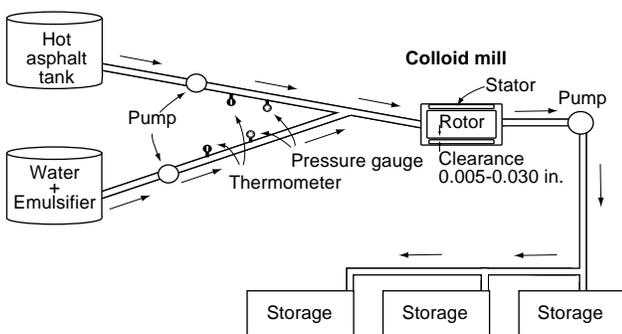
**Figure 2. Manufacture of emulsified asphalt**
