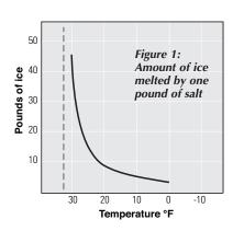
cantly. Figure 1 shows that salt can melt five times as much ice at 30°F as at 20°F. Small differences in pavement temperatures have a noticeable effect. Truck mounted temperature sensors give operators information to make better application decisions.
