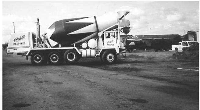
Another factor is the amount of weight and number of tires on each axle. Damage increases rapidly with higher axle loads and actually worsens at a faster rate than the load increases. A nine-ton axle load, for example, causes about ten times more damage than a five-ton axle load. Distributing a vehicle's weight and its payload over more axles and tires makes the load lighter at each point of contact, reducing damage to the road.
