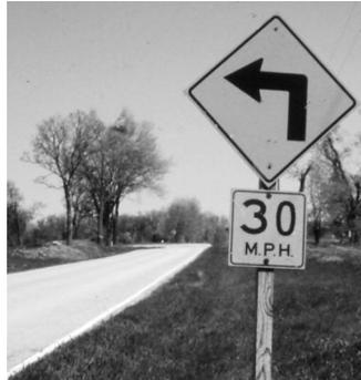
two-lane highways in the study, posted advisory speeds at most curves were well below prevailing traffic speed, and below speeds established using recommended devices and criteria.
