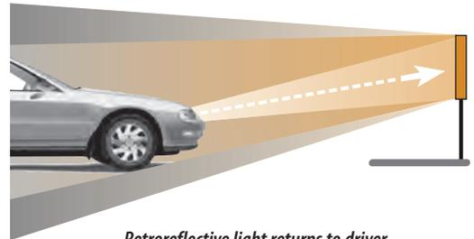
Retroreflective light returns to driver from headlight beam striking road sign.
